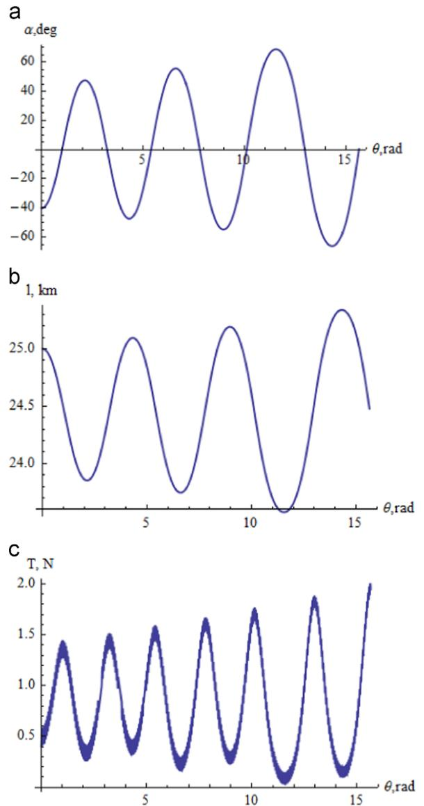
**Fig. 2.** The dependence of the deflection angle  $\alpha$  from true anomaly (a), the dependence of the tether length from true anomaly (b), the dependence of the tether tension from true anomaly (c).
